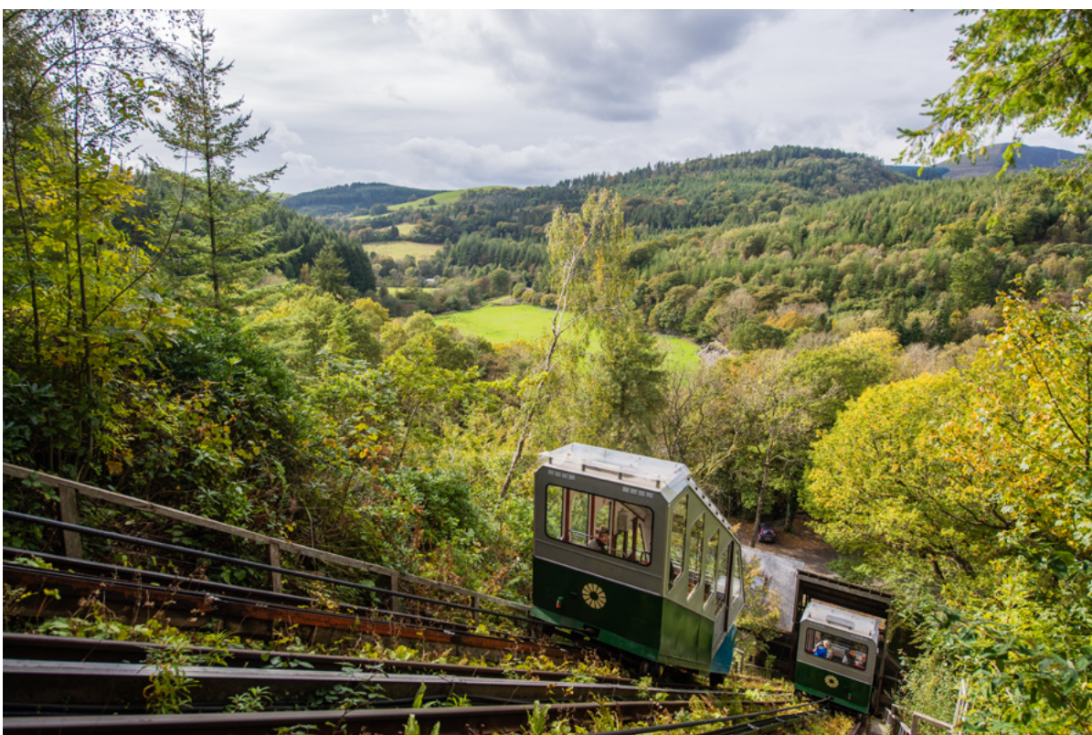
The water-balanced funicular railway takes thousands of visitors up to CAT’s visitor centre from March to October.
